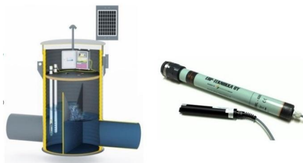
Figure 10. On the left, EHP-Monitoring Station for water flow and quality monitoring in arctic field conditions can measure several parameters online, such as water flow/level, pH, EC, Eh, DO, \text{NO}_3^- -N, \text{NH}_4^+ -N, T, COD, TOC, solids, and turbidity. On the right, a portable water level and quality monitoring device for wireless monitoring of groundwater and surface water level and quality in the field. Depending
